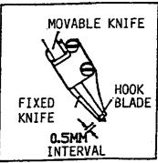
WHEN MOVABLE KNIFE MOVE TO ITS UPPERMOST IDEAD POINT, THE FRONT EDGE OF THREAD CLAMP SPRING AND MOVABLE KNIFE SHOULD BE EVEN. AND THE FRONT EDGE OF KNIFE PRESSURE SPRING AND FIXED KNIFE SHOULD BE EVEN.
